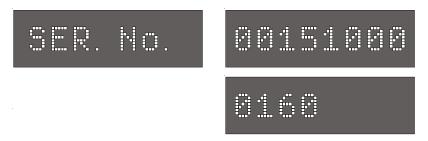
The most significant eight digits of the serial number are displayed first, after pressing the Set button the last four digits are shown.
